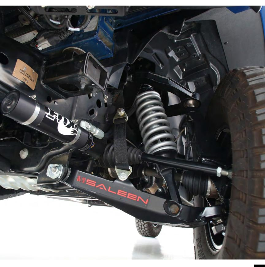
THE FRONT SUSPENSION SYSTEM FEATURES SALEEN'S Control Arms Matched With a New Steering Knuckle and Custom Tuned Fox 2.5 coilover Shocks
