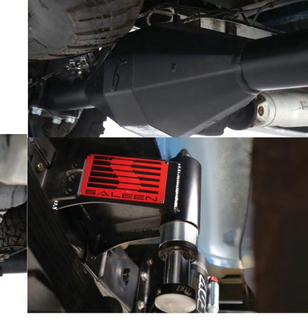
At the rear Saleen uses its own design of leaf springs, and added Fox bump stop with frame gussets to create 14-inches of travel. This is all connected to a fullfloating rear axle and heavy-duty housing that is only available in the Saleen "Black Label" version of the truck, which adds the highest performance level and output available on the truck. White and Yellow Label models are also available with fewer options.
