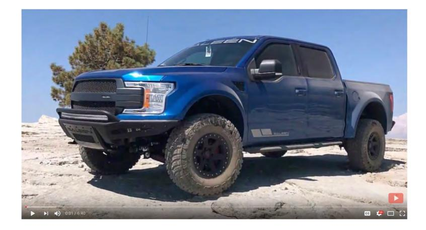
The front and rear tube bumpers are wider to match the flares and integrate Rigid LED lighting, while a large skid plate is added to the front with the Saleen logo cut out. Foutz worked with Saleen designers to create the truck's rock sliders and they also feature integrated lighting for a unique appearance.
